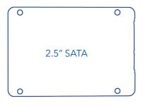
(The 2.5-inch designation actually refers to the size of a typical laptop drive platter, the disc inside the housing that data is actually recorded on.)
